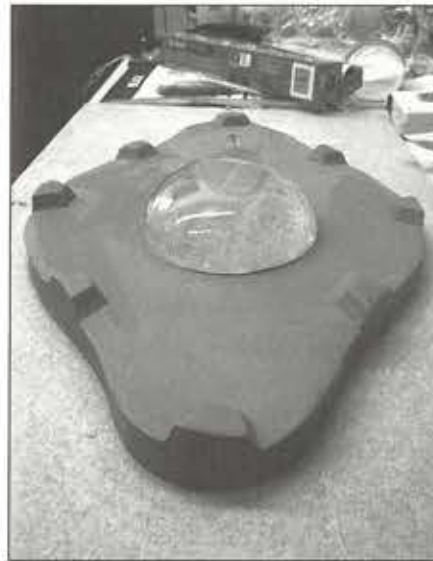
Clay bed with a diameter that allows for the core, thickness of glass, and the mold wall.
